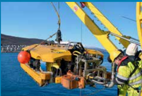
The Framo ROLS is prepared to enter the water
