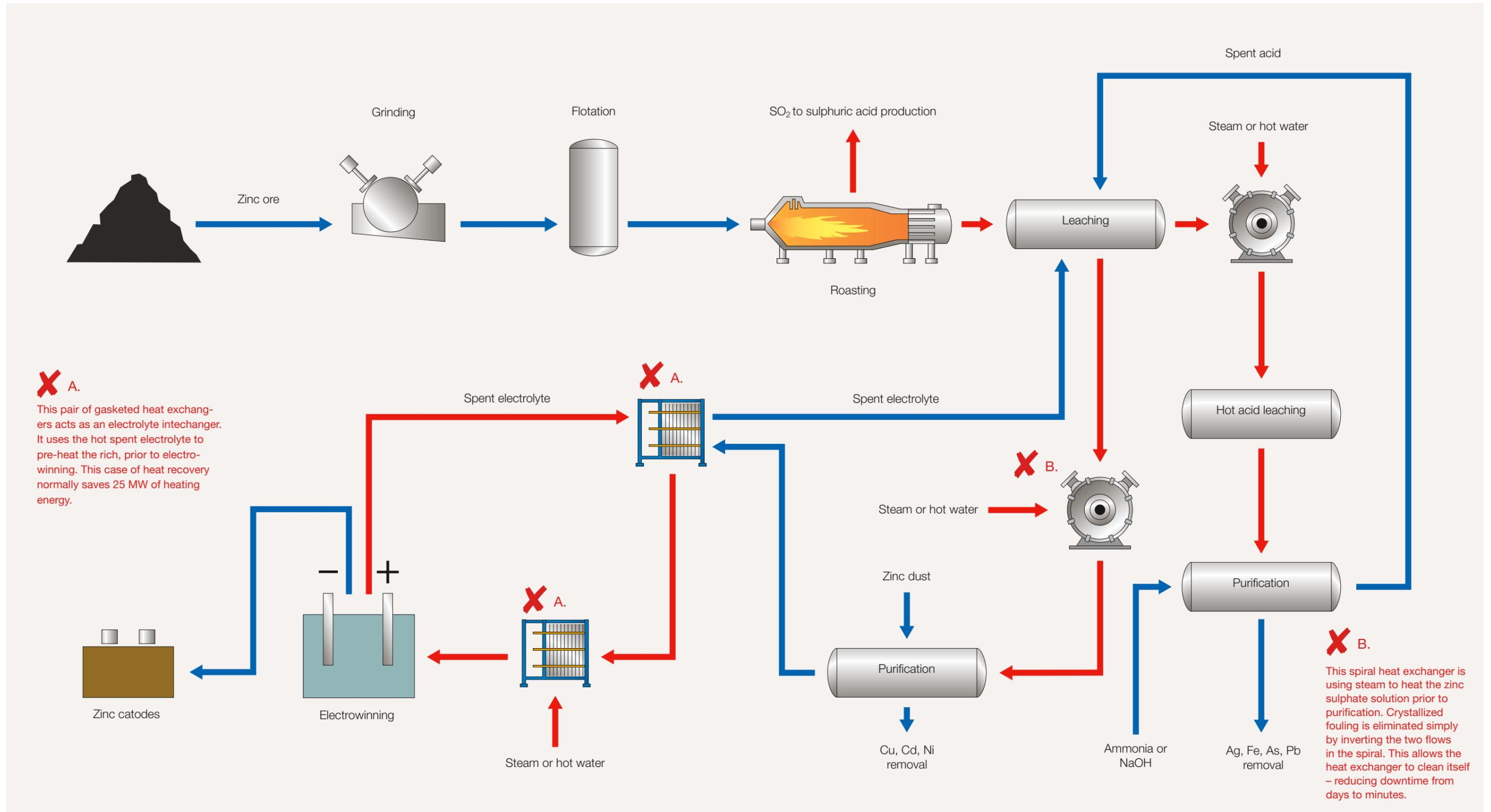
In zinc production, roasting, leaching, electrowinning and other energy-intensive extraction processes can be tapped for vast amounts of heat. Heat that can be fed right back into the flow, with an unparalleled yield.
