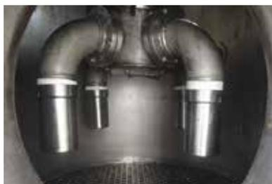
The larger hole size compared with a platter distributor reduces the risk of blocking the nozzle and ensures even distribution to the tubes.
