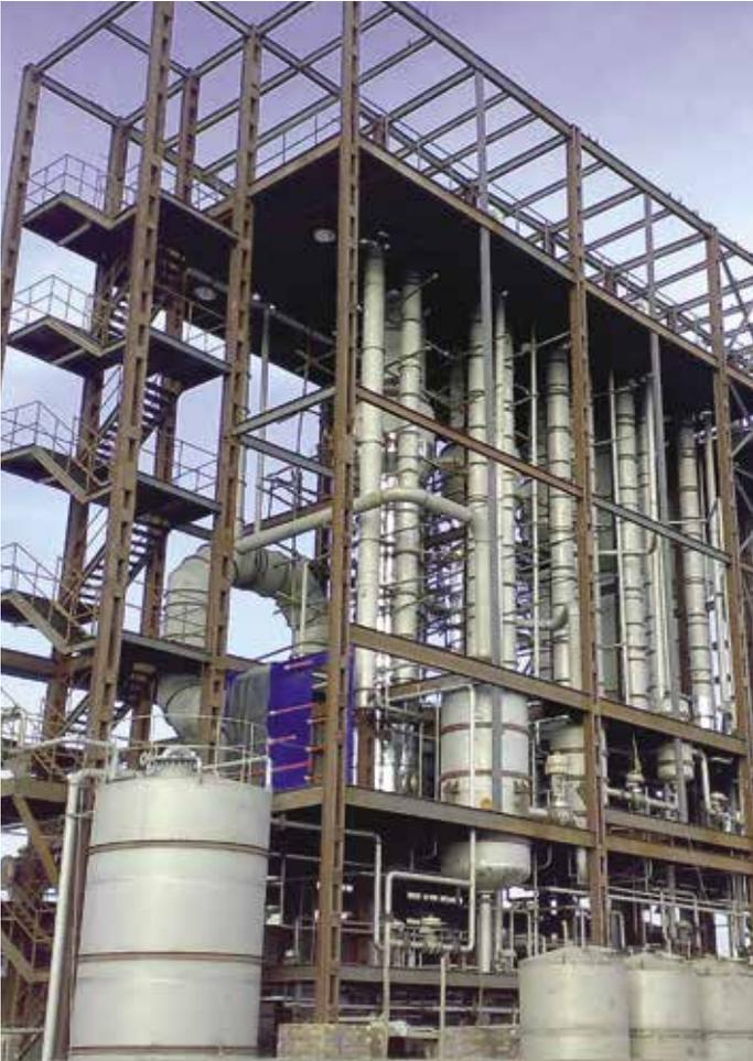
The right configuration and the ideal combination of Alfa Laval FilmVap evaporators and forced-circulation evaporator provide reliability as well as savings on both energy and cleaning in certain applications that include vinasse.
